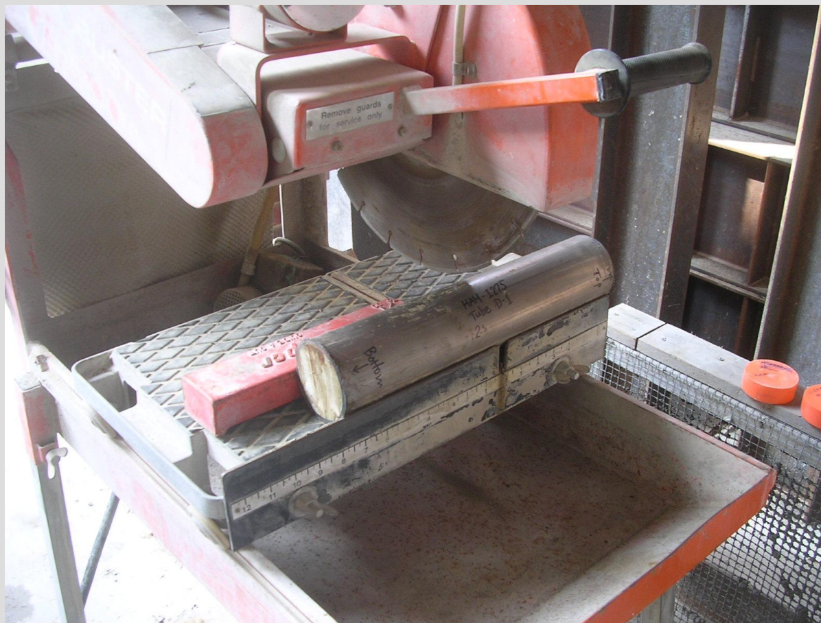
Cutting of Shelby Tube into Shorter Sections
