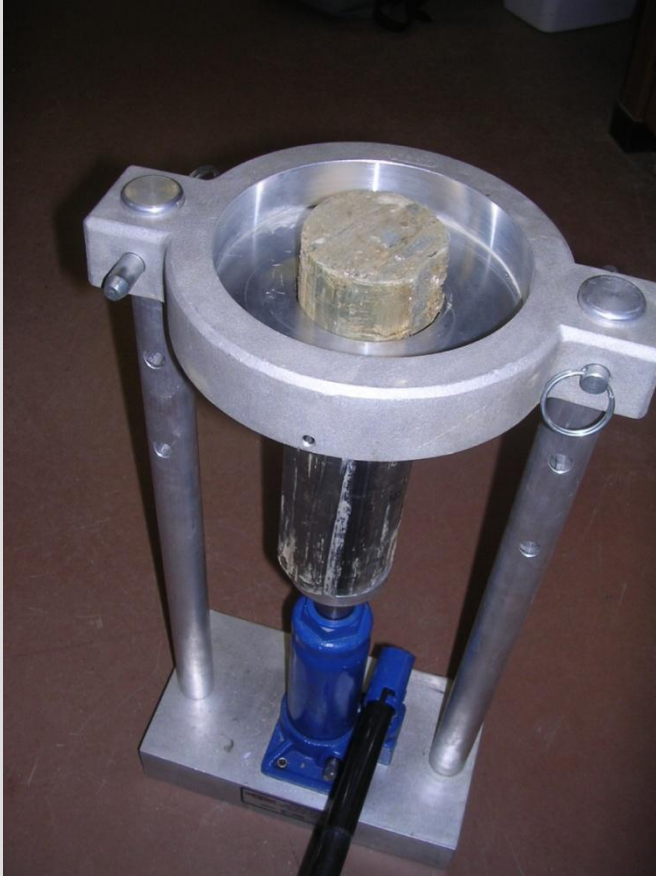
Hydraulic Jacking of Soil Sample
